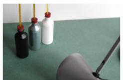
• Set your data logger to take readings every second and switch on the lamp. Typical results are shown below. If you have a fourth probe you could use it to monitor the room temperature.
